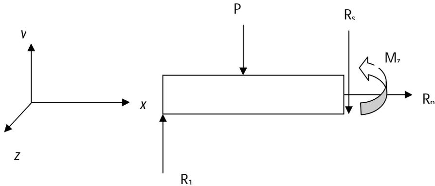
Considering static equilibrium with upward acting forces and clockwise moments being positive rise have for the whole beam:
