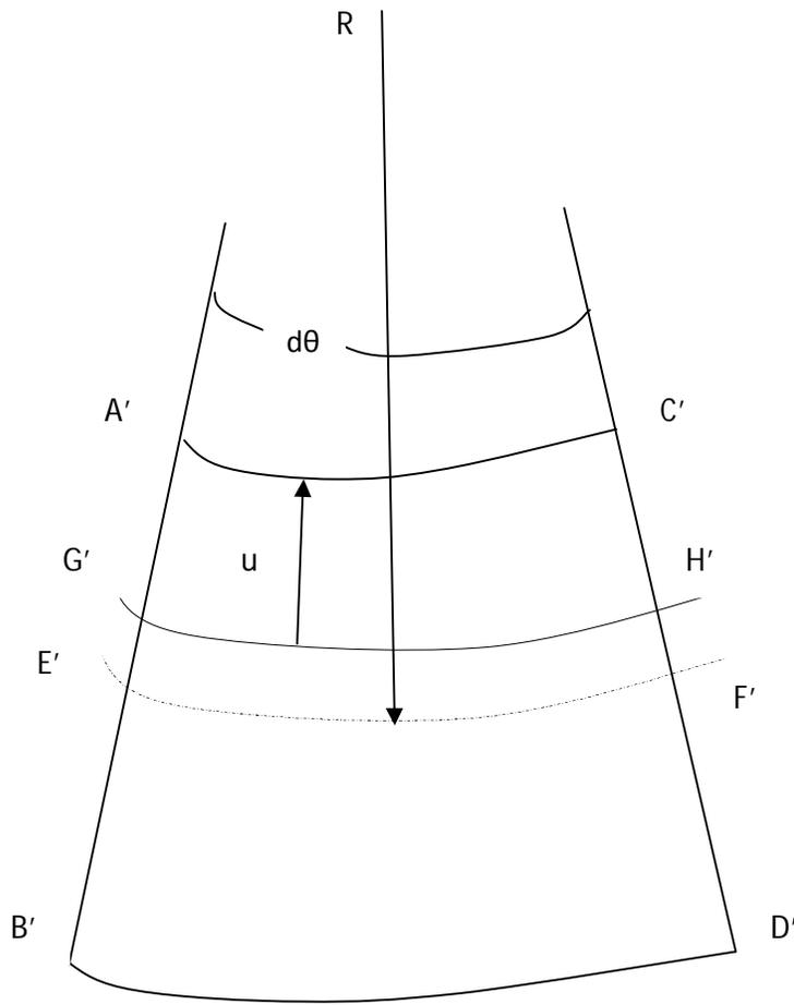
$u$  represents the distance between the neutral axis  $EF$  and some other parallel line  $GH$  in the plane of symmetry. We assume that the distance between these lines in the deformed beam will not be significantly different from the original distance in the unloaded beam.
