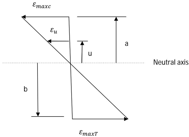
The strain at any point at a distance  $u$  from the neutral surface can be determined by the simple ratio:
