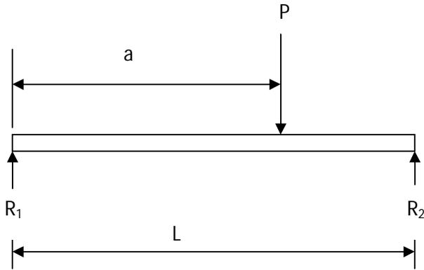
Equilibrium of forces in the vertical direction with upwards acting forces being positive gives;
