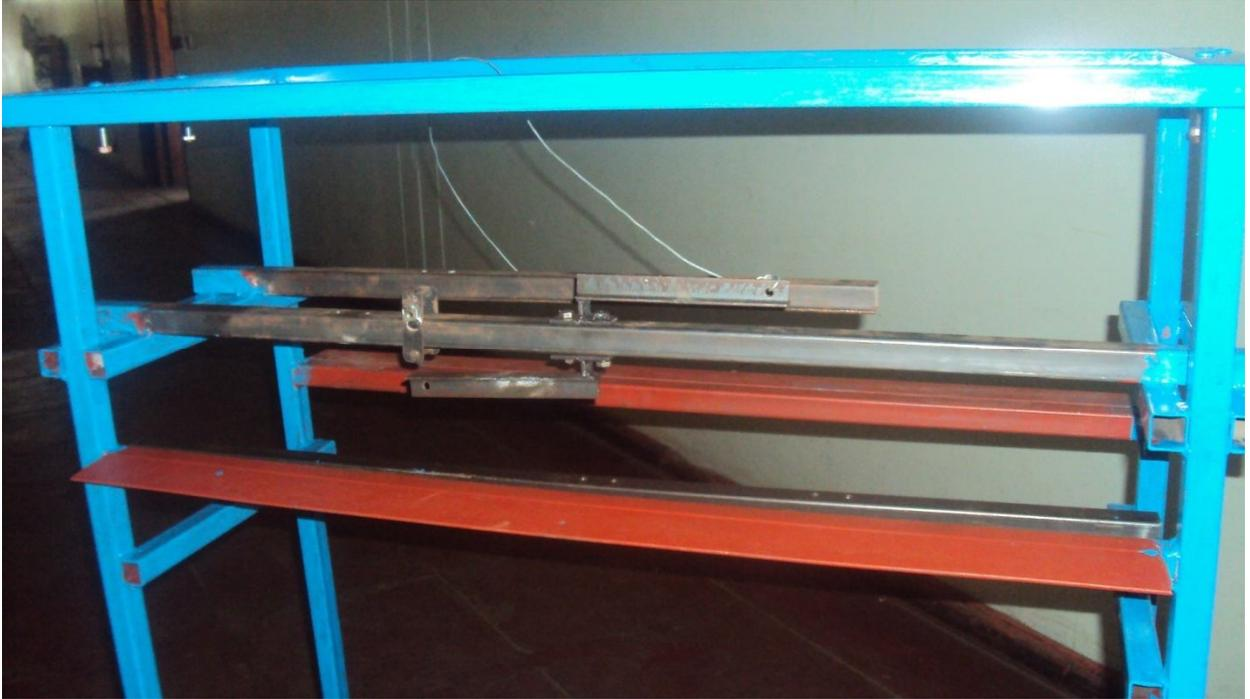
Beams with loading fixtures
