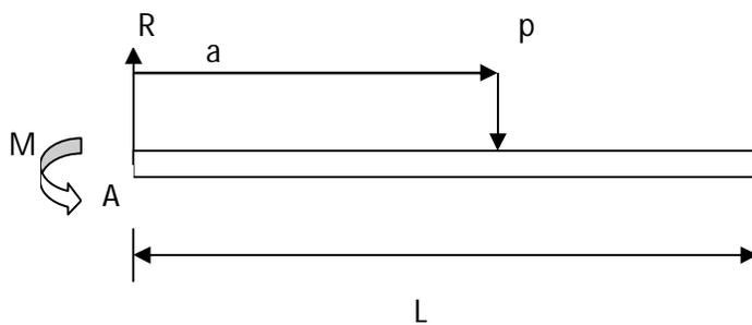
Equilibrium of forces in the vertical direction with upwards acting forces being positive gives;
