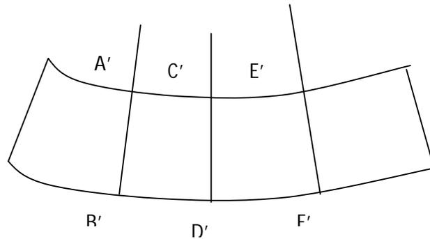
The portion of beam between plane sections AB and CD was originally geometrically identical in length and cross section with the portion between sections at CD and EF. Also each of these portions is loaded in exactly the same manner that is by couples. Therefore in order that each of these portions may be geometrically compatible in the deformed state, we may logically expect that these portions would undergo similar deformations.
