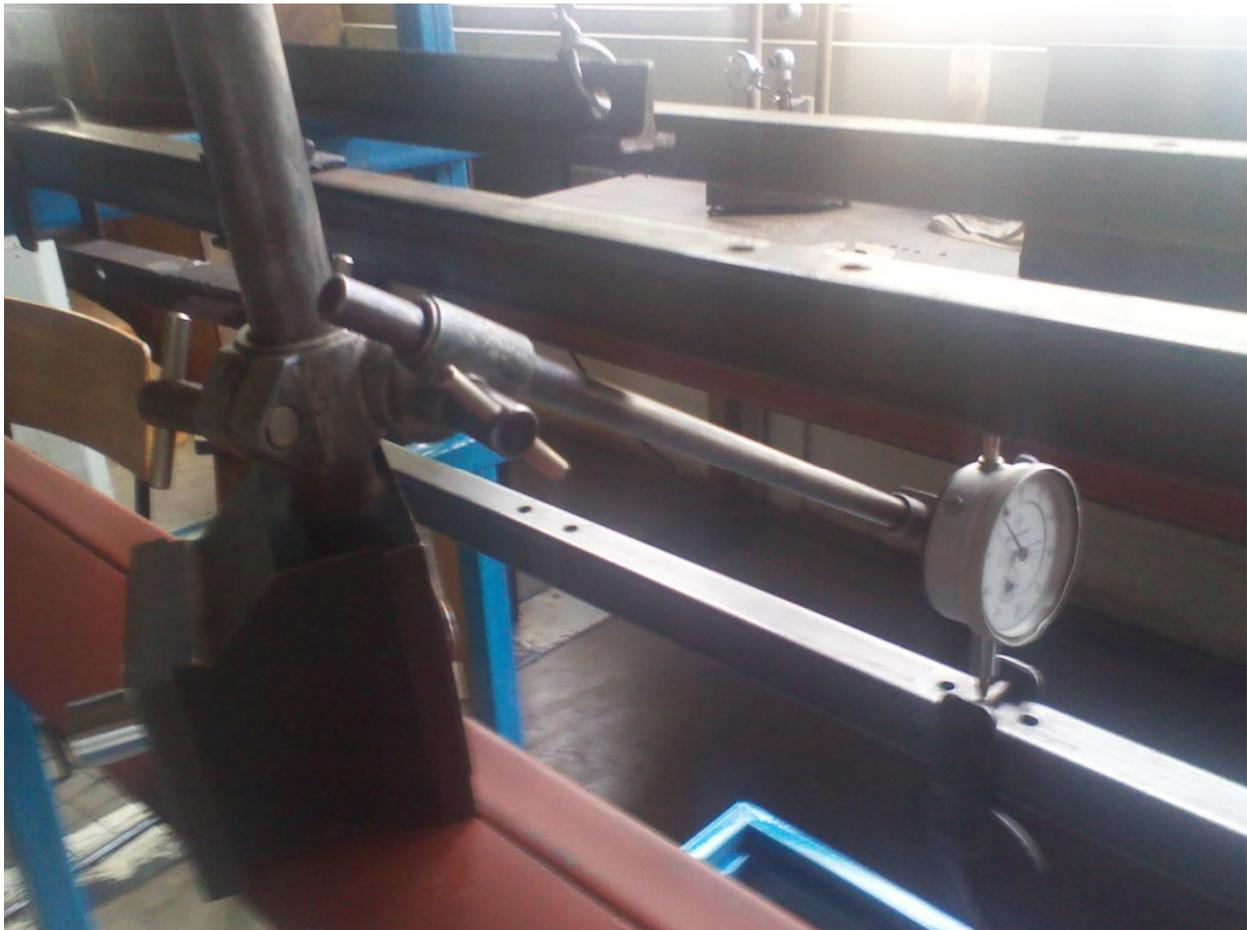
*Experimental deflection for simply supported beam with central point load.*
