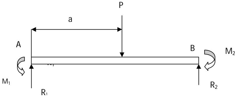
Equilibrium of vertical forces with upward acting forces being positive i.e.
