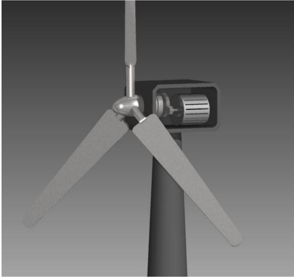
Fig 9.2: Inventor Software simple Diagrammatic representation of a three bladed wind turbine with an alternator.
