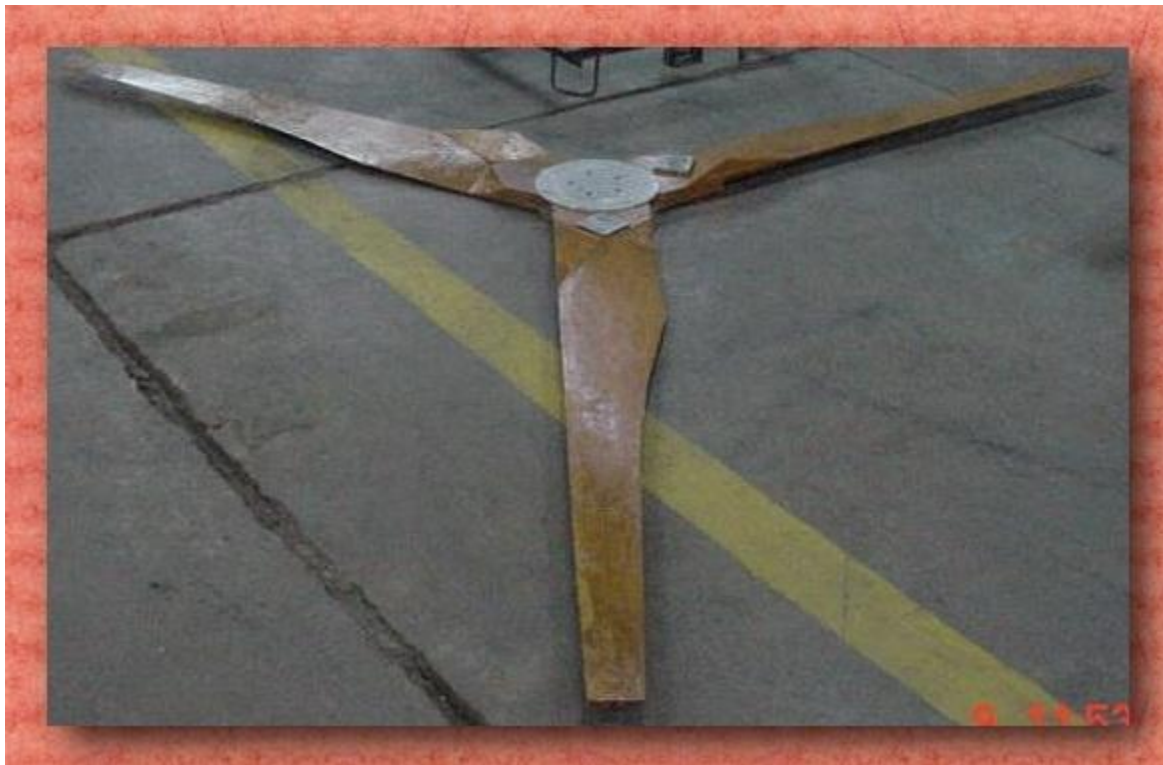
Fig 6.3: A sample diagram showing a three bladed aerofoil (Horizontal axis wind turbine) (Ref. 5)
