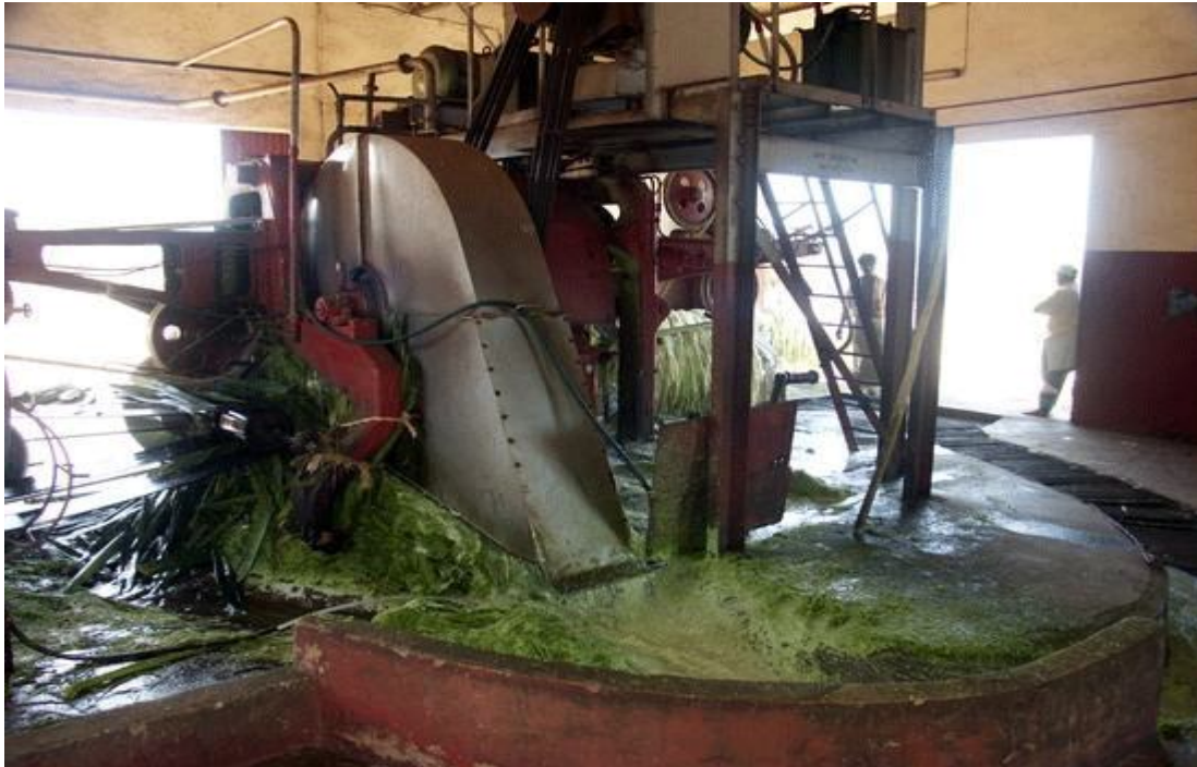
Fig. 3.6 Automatic sisal decorticator
