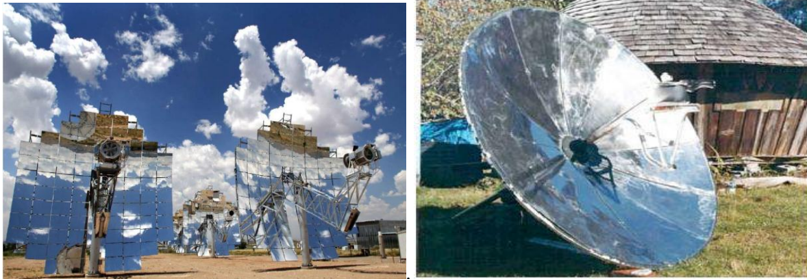
Figure 2.10: Examples of parabolic reflectors
