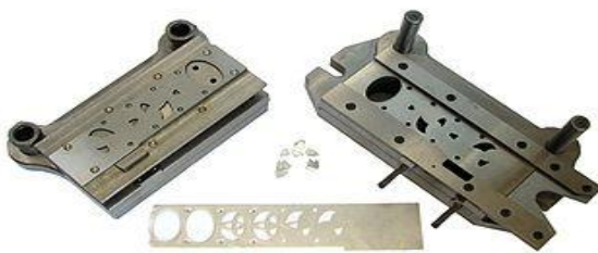
Fig 2.3.16: Progressive die with scrap strip and stampings
