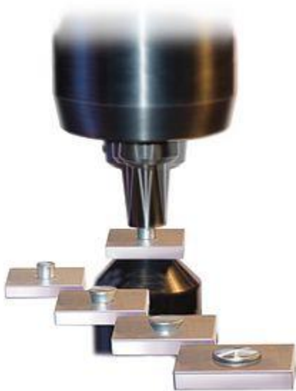
Fig 3.3.3: Example of a 4-step orbital rivet en.wikipedia.org/wiki/riveting_machines
