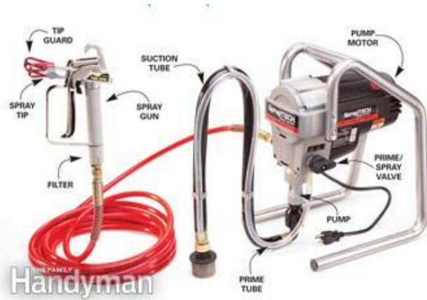
Fig 3.4.13: Parts of airless sprayer
