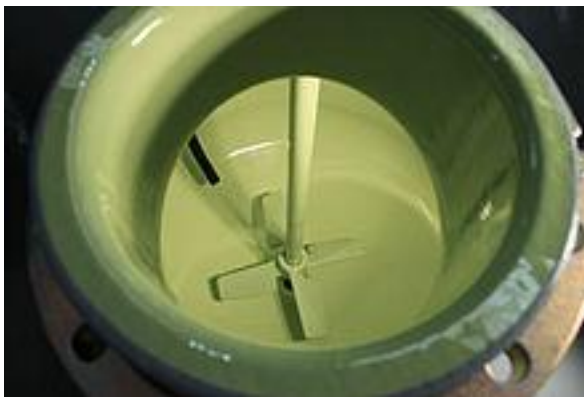
Fig 3.4.16: The porcelain-enamelled interior of a chemical reaction vessel
