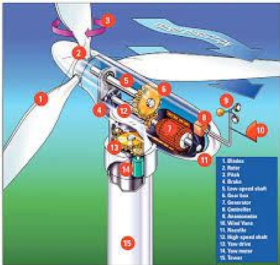
Figure 1.0: Components of a conventional wind turbine ( http://www.flickr.com/photos/pjh/185488411/ .)
