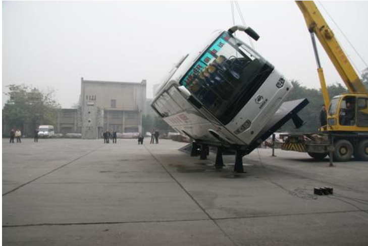
Figure 2.7-2: A tilt test set up (Courtesy: www.eobus.com )
